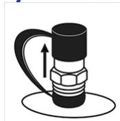
If the regulator on/off switch gets stuck when turning the supply on, it means that the regulator has been connected incorrectly. In this event the regulator must be disconnected and the correct steps to reconnect repeated from the beginning
