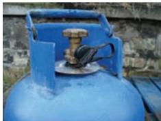
1. **Never** disconnect the Regulator (or connecting nut) with the valve open
