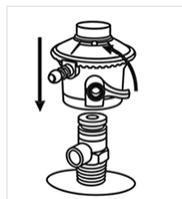
1. Turn the orange cap so that the arrow is pointing to the gap in the shroud
