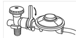
7kg, 12kg and 15kg Butane Cylinders have a 21mm valve and must only be used with a 21mm regulator
