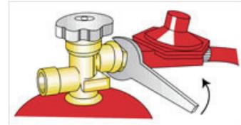
**Reminder:** Propane cylinders have a 'female' valve connection. Check the connection is clean and undamaged. This is a 'face to face' deal and requires the correct size spanner and is to be fully tightened. (left hand thread).
